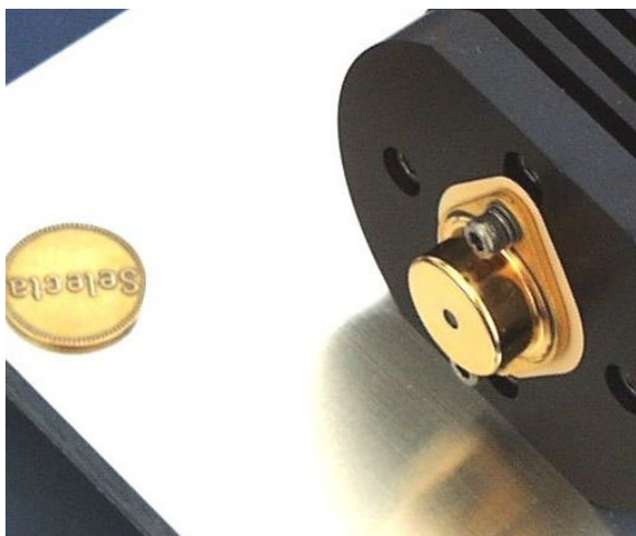
Figure 2. Microchip laser system, installed into a standard TO-3 package. This is a commercially available passively Q -switched Nd:YAG laser operating at 1064 nm (Poly-Scientific ML-00040).
