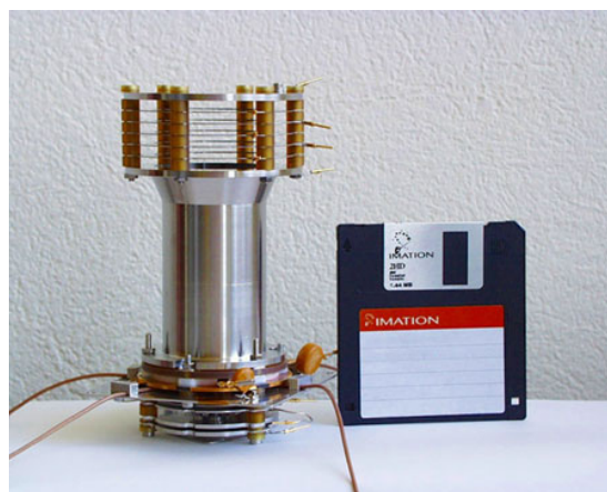
Figure 4. Laboratory prototype mass analyser v1.0. At the top of the image are the plates defining the reflectron. The flight tube is visible in the centre of the picture, and at the bottom are shown the ion optics that would be adjacent to the surface to be sampled. The dimensions are 150 mm in height, and 60 mm in diameter, i.e., about the size of a soda can.
