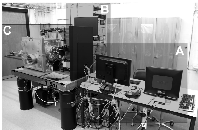
Figure 1. Overview of the instrument setup in the laboratory. (A) represents the remote control station; (B) the electronic equipment, e.g. measurement computer, power supplies, etc.; (C) the instrumental setup itself. Detailed information about part (C) can be found in Fig. 2. The argon sputter gun is not visible in this figure due to maintenance.
