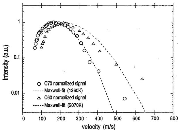
FIG. 4. Velocity distributions for laser desorbed neutral  $C_{60}$  and  $C_{70}$ . Dashed curves give best fits of Maxwell-Boltzmann distributions with the measured data.
