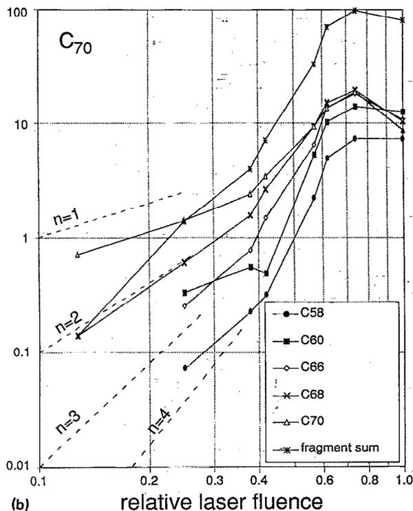
FIG. 3. Dependence of the ionization and the fragmentation on the laser intensity for  $C_{60}$  (top panel) and  $C_{70}$  (bottom panel). Relative laser fluence of 1.0 corresponds to  $40 \text{ mJ/cm}^2$  and  $110 \text{ mJ/cm}^2$  for  $C_{60}$  and  $C_{70}$ , respectively. Sum of fragments extends from  $C_{34}$  to  $C_{38}$  for  $C_{60}$  and from  $C_{42}$  to  $C_{68}$  for  $C_{70}$ .
