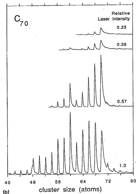
FIG. 2. Mass spectra of postionization and fragmentation of neutral  $C_{60}$  (top panel) and  $C_{70}$  (bottom panel) laser desorbed from a copper substrate. Relative laser fluence of 1.0 corresponds to 40  $\text{mJ}/\text{cm}^2$  and 110  $\text{mJ}/\text{cm}^2$  for  $C_{60}$  and  $C_{70}$ , respectively.
