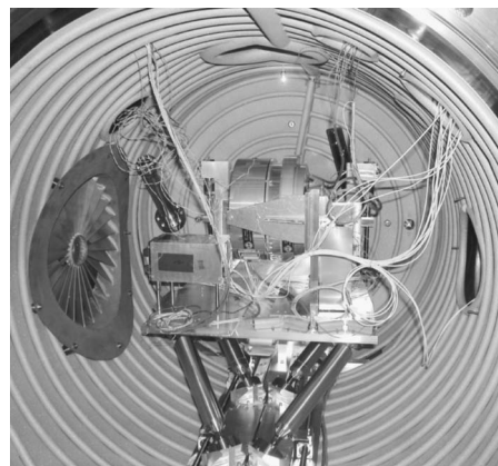
FIG. 12. IBEX-Lo prototype (cylindrical structure in the center) installed in the MEFISTO calibration facility of the University of Bern, Switzerland. The ion beam enters the chamber from the left through the fan-shaped opening. The ion beam is neutralized in the box left of the center of the image (Ref. 28) prior to entering the IBEX-Lo prototype. Most electrostatic shielding around the prototype setup was removed for this picture.
