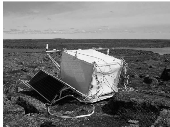
Fig. 6. MEAP on ground near Umingmaktok, Canada, at 67.17 N/105.15 W. Whereas the solar panels are crashed (being part of the crashable structure), the main platform is virtually undamaged. The platform continued transmitting data after touchdown.
