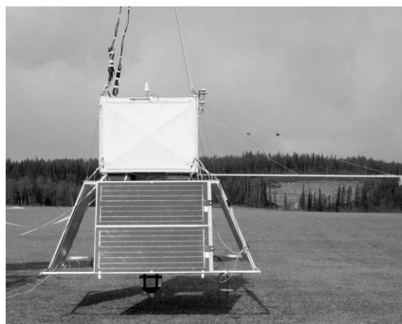
Fig. 1. MEAP gondola during a test on the balloon launch pad. The payload is contained in the white box mounted on top of the solar panel structure. The boom going to the right holds at its end the gas inlet filter of P-BACE (not visible). The gondola with solar panels is about 4 m in height.
