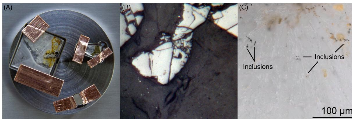
**FIGURE 1** (A) Samples are placed on a stainless-steel holder, in cavities, and stabilized by a cooper tape for UHV applications. (B) Sample material that contains the trevorite mineral (black area). White patches contain mostly the mineral spinel. (C) Aragonite host material (bright material) containing micrometer-sized inclusions (in black)
