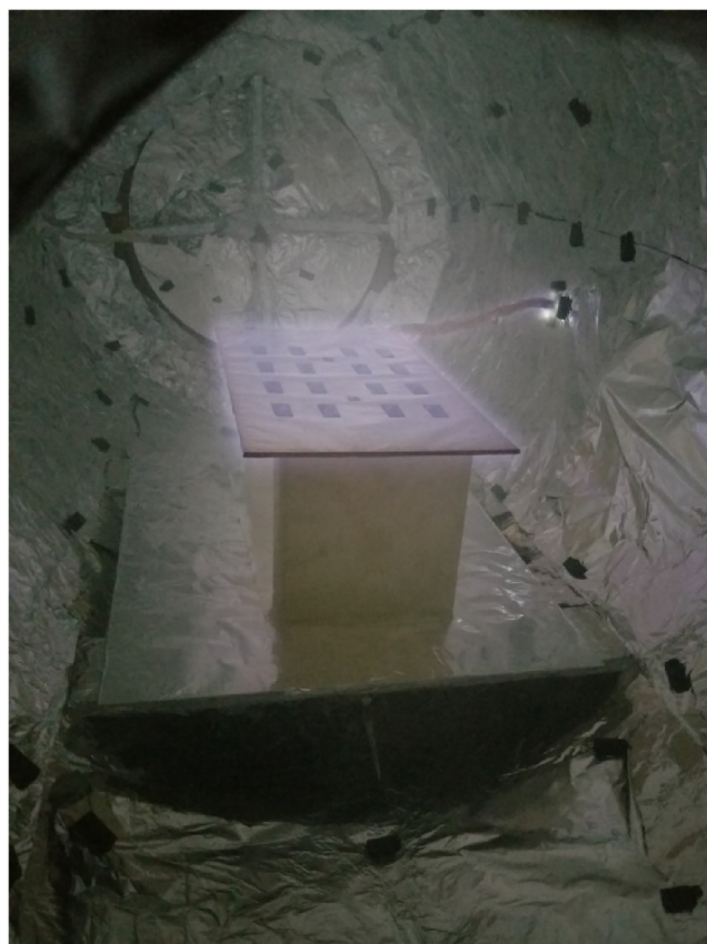
FIG. 5. Holding plate with conversion surface substrates during the deposition process.
