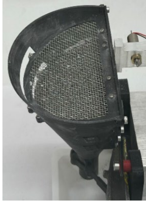
Figure 9: 3D printed funnel with 63^\circ wall angle used to test and validate the sieving performance.
