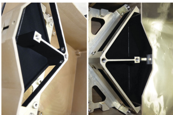
Fig. 56 HEP-ele detector section structures blackened with conductive paint
