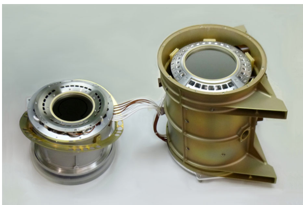
Fig. 41 Copper sulfide blackened energy analyzer (left) and entrance section (right)
