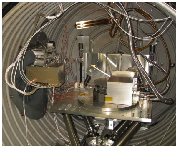
Fig. 81 ENA at the MEFISTO calibration facility. The neutral beam is emitted from the beam neutralizer on the left (gold box). ENA (center) is encapsulated in thermal insulation sheets to facilitate temperature control. The entire instrument setup can be moved and rotated relative to the incoming neutral beam with 6° of freedom
