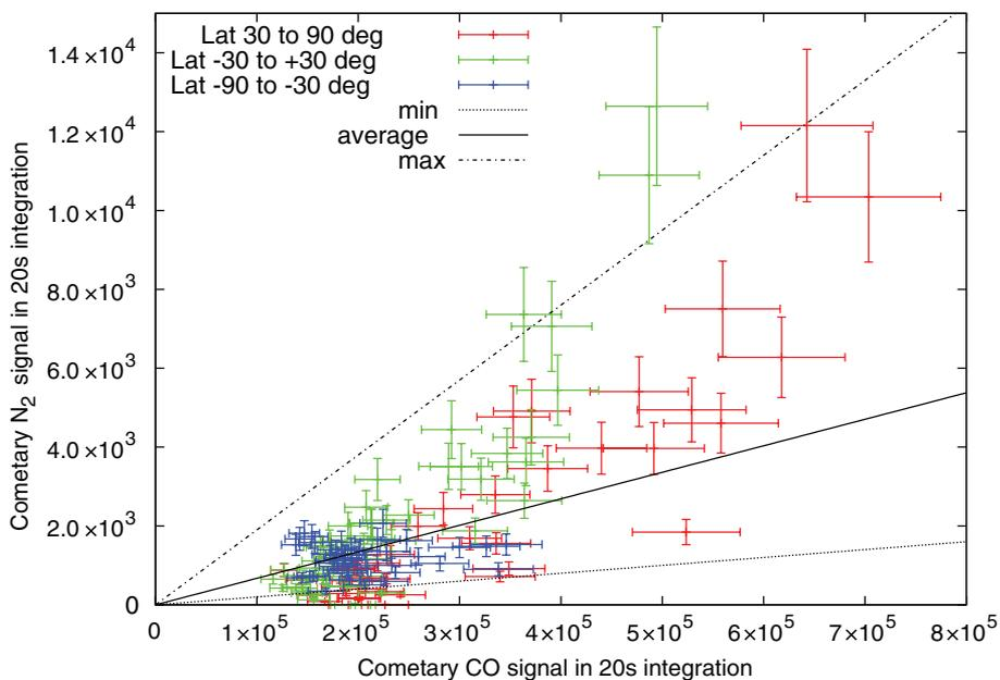
**Fig. 3. Cometary parent  $N_2$  versus CO signal.** The min and max lines bracket most measurements. To derive the  $N_2/CO$  ratio, the detector signal ratio in the plot has to be divided by the differential sensitivity of 1.175. The average  $N_2/CO$  ratio of  $5.70 \times 10^{-3}$  is given by the solid black line; the min and the max lines show the observed variation and correspond to ratios of  $1.7 \times 10^{-3}$  and  $1.6 \times 10^{-2}$ .
