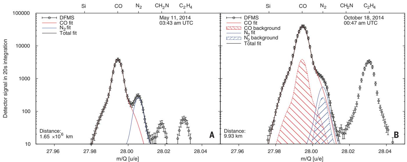
**Fig. 1. Mass per charge 28 u/e spectra before (A) and after (B) entering the coma of 67P, including statistical and 10% pixel gain error.** (A) was obtained in May 2014 and (B) is a representative spectrum from October containing the sum of the cometary parents and fragments and the spacecraft background signals.
