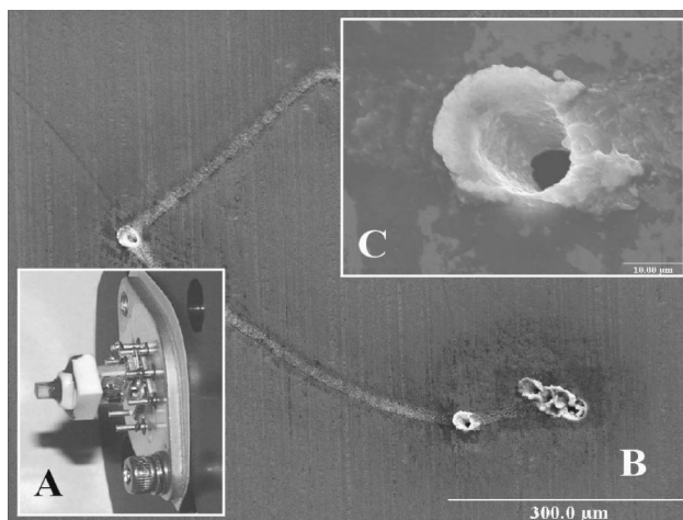
FIG. 2. (a) Microchip laser system in a TO-3 package with housing removed. This is a commercially available passively Q -switched laser operating at 532 \text{ nm} (Synoptics ML-00039). (b) Craters from laser shots into a piece of aluminum moved across the focus of the laser beam. (c) Magnified image showing a laser-drilled hole with a diameter of about 15 \mu\text{m} .
