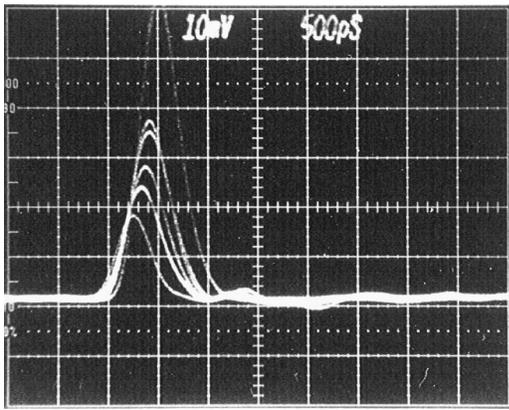
FIG. 5. Optical impulse after the optical converter (Newport, model AD-200) recorded with a 1 GHz analog oscilloscope with the horizontal scale being 500 ps/div and the vertical scale being 10 mV/div. The detector configuration is: three MCPs, no spacer rings,  $U_{\text{MCP}} = -3800$  V,  $U_{\text{bat}} = 1.5$  V.
