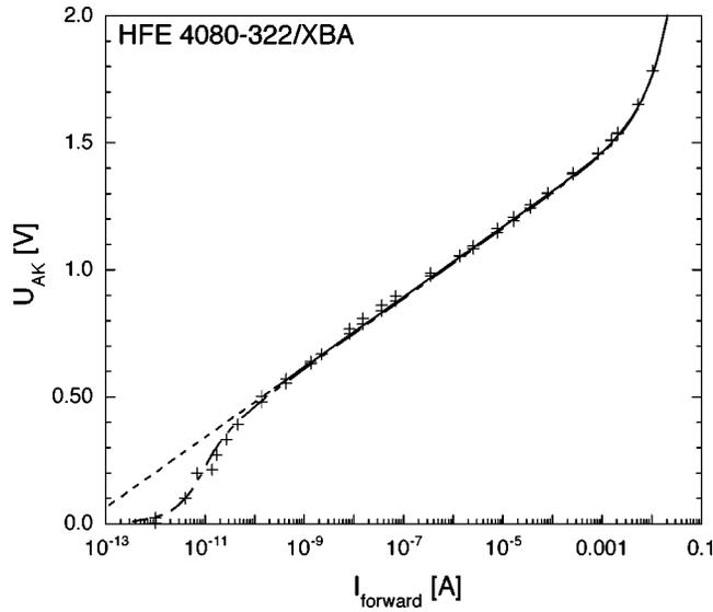
FIG. 3. Symbols give the measured voltage–current relationship of the used VCSEL (model HFE4080-322/XBA, Honeywell). The current was measured with an electrometer (Keithley, model 6517A). The solid line is a fit with the usual exponential relationship and a series resistor [Eqs. (5) and (6)], and the dashed line is the extension to lower currents where the model does not fit the measured data. The dash-dotted line gives a fit with an additional parallel resistor.
