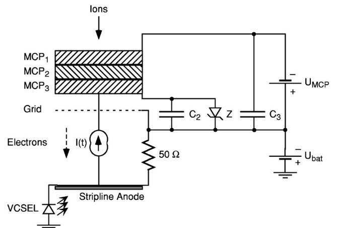
FIG. 2. Schematics of the detector electronics accommodating the laser diode. Details of the circuits have been given before (see Ref. 4).
