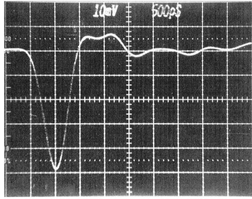
FIG. 1. Electrical performance of the original MCP detector with a matched pair of channel plates (Photonics, model G6-25-SE/ST/6/A) and without a spacer ring between the two plates. The measurement was made using a 1 GHz analog oscilloscope with the horizontal scale being 500 ps/div and the vertical scale being 10 mV/div. The front MCP voltage was  $U_{\text{MCP}} = -2700$  V and the anode was at ground potential.
