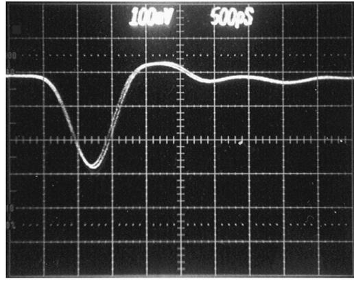
FIG. 4. Electric impulse at the anode recorded with a 1 GHz analog oscilloscope at  $50 \Omega$  input resistance with the horizontal scale being 500 ps/div and the vertical scale being 100 mV/div. The detector configuration is: three micro-channel plates, no spacer rings,  $U_{MCP} = -3800$  V,  $U_{bat} = 0$  V.
