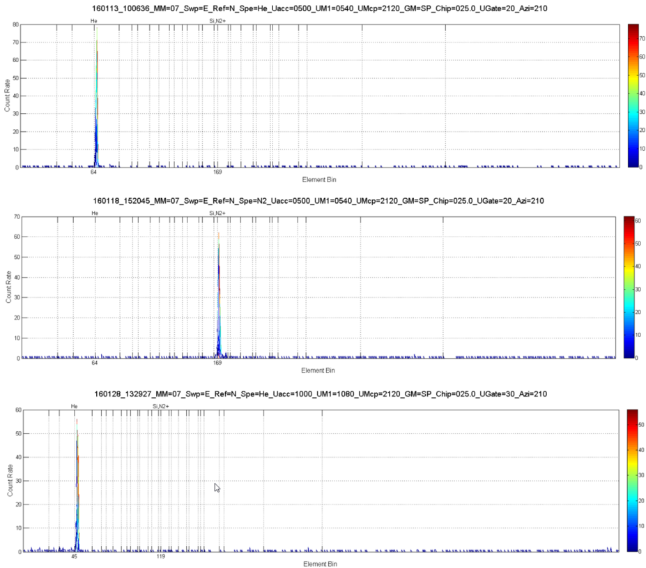
Fig. 81 ToF spectra in single pulse mode for two different species ( \text{He}^+ , \text{N}_2^+ ) obtained at 500 (upper panels) and 1000 eV (lower panel)
