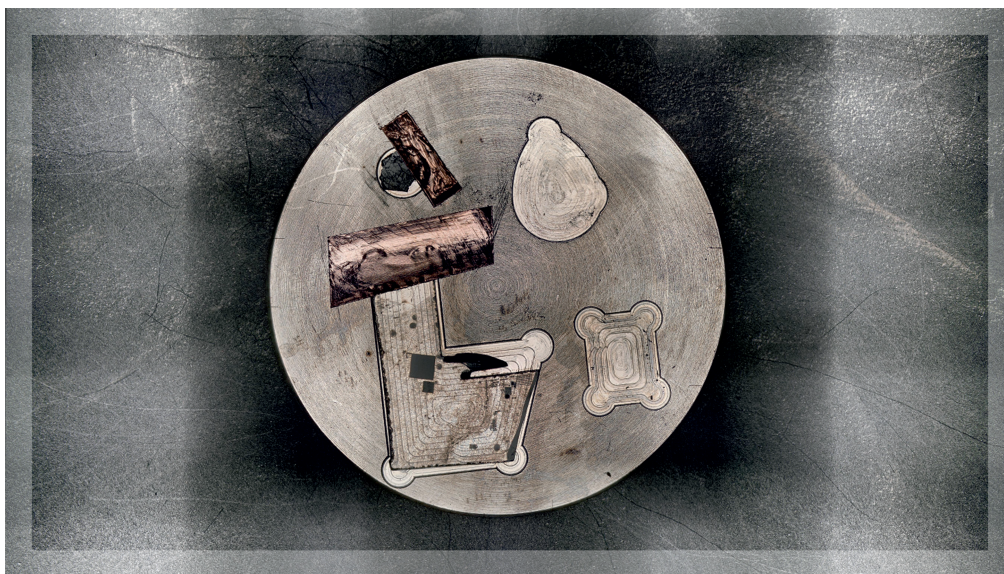
FIG. 1. Panoramic image of the Gunflint chert thin section mounted on a steel holder (L-shaped sample, left bottom). Color images are available online.
