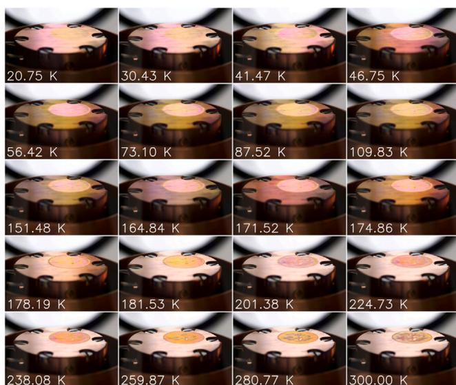
Fig. 11. Evolution of an  $\text{CH}_4\text{:H}_2\text{O:N}_2$  ice that has been irradiated for 4 h during the TPD. The desorption of various molecules can be clearly seen in the color change on the sample holder. A brownish residue remained on the sample holder after the TPD was completed. (For interpretation of the references to color in this figure legend, the reader is referred to the web version of this article.)
