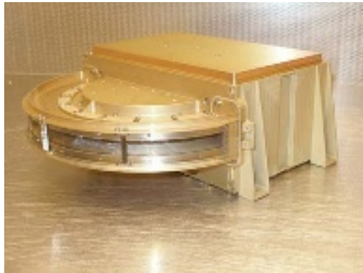
Figure 2. Photograph of the prototype of the instrument. The collimator and the wave-type structure are on the left-hand side, and the TOF part, the MCPs and the front-end electronics are inside of the box on the right side.
