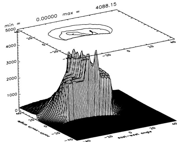
Fig. 3 Neutral oxygen flux levels at  $x = -1.29$ ,  $y = -0.72$ ,  $z = 0.09$ . For comparison, the contours for the angular flux distribution are shown in the top of the figure.
