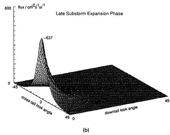
Fig. 8 Neutral hydrogen fluxes with energies below 1 keV derived from (a) a late substorm growth phase equilibrium and (b) a substorm growth phase expansion state model by 3-D resistive magnetohydrodynamic simulations. In either case, the spacecraft location is assumed to be  $x_{SM} = -5 R_e$ ,  $y_{SM} = -0 R_e$ , and  $z_{SM} = 8 R_e$ . Shown is the variation of the flux with crosstail and downtail look angles.
