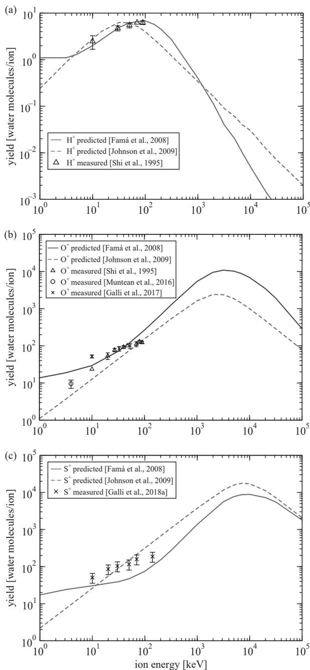
**Figure 15.7** Ion sputtering yields for an ice temperature of 100 K and an incidence angle of  $45^\circ$  including semi-empirical formulae by Famá et al. (2008) (blue solid curves) and by Johnson et al. (2009) (red dashed curves) and some experiment results (Shi et al. (1995); Muntean et al. (2016); Galli et al. (2017, 2018b), black symbols) for  $H^+$  (a),  $O^+$  (b), and  $S^+$  (c).
