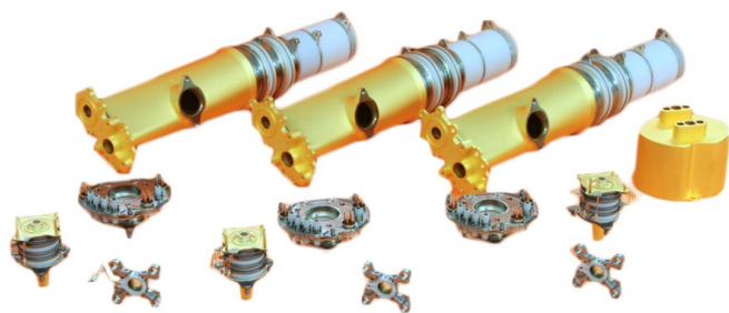
Figure 3. PFM, EQM and FS of the drift tube assembly with ceramic-metal ion mirror (top) and ion source (bottom).
