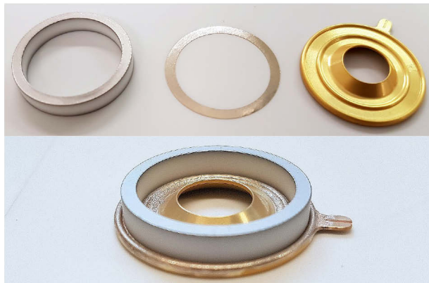
Figure 5. First brazing test (AL 300 MET (Ø24 x Ø20 x 4) + Incusil ABA + Mo85Cu15 (TiAlN/W/Cr+Au)).
