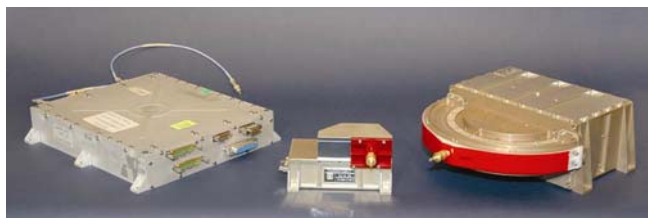
Figure 1. SARA flight model. From left to right are shown the Digital Processing Unit (DPU), the Solar Wind Monitor (SWIM), and the Chandrayaan Energetic Neutrals Analyser (CENA).
