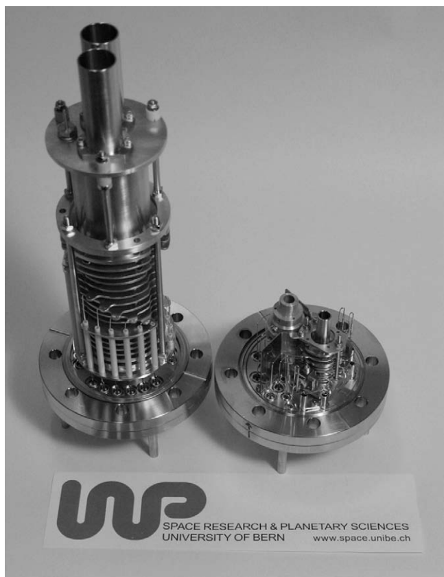
Fig. 2. The two CF-63 flanges of the P-BACE sensor: on the left side the reflectron with drift tubes, on the right side the ion source and the detector.
