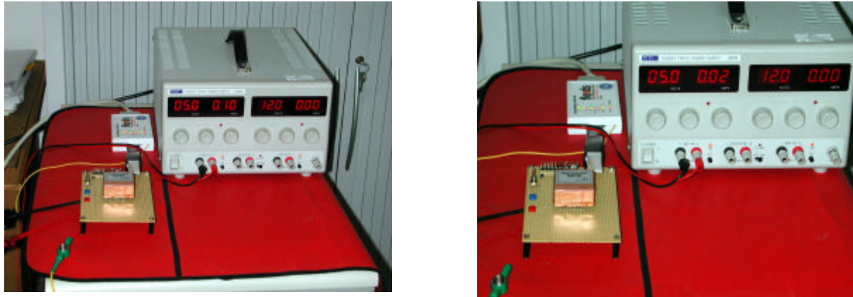
Figure 12. Right panel: uDPU in stand-by (100mW on primary). Left panel the uDPU during memory test (500 mW on primary).
