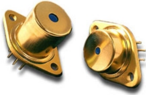
Figure 5. Microchip laser systems in a TO-3 package. This are commercially available [6] passively Q-switched lasers operating at 532 nm (on the left: Synoptics ML-00039) respectively 1064 nm (on the right: Synoptics ML-00040).
