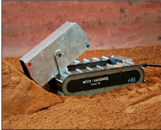
Figure 3. Prototype rover “Nanokhod” for the Bepi-Colombo mission, designed and built by “Von Hoerner & Sulger GmbH”, Germany (with permission).
